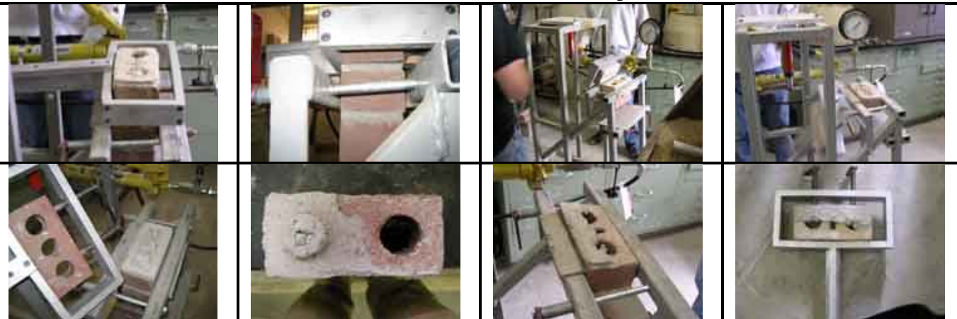
Bond Wrench Test Failures
