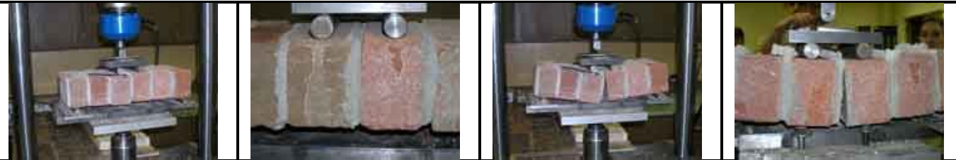
Four-Point Bending Test
